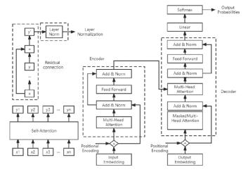
Figure 2 Transformer Flowchart.
